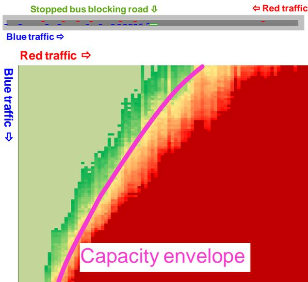
Figure 3: Ensemble modelling output. Green to red shows good/bad network operation.
